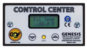
temperature will start changing in that direction in tenths of degrees. Keep in mind that thermometers can be off or change over time and should not be relied upon initially. The quality of hatch may be the best indicator as to the temperature setting after considering other factors that can affect the hatch (please see the Poor Hatch section on the last page).
